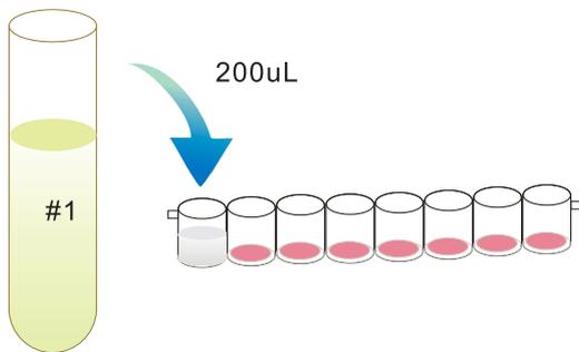
3. Take 200ul sample into the wells using pipet. You can also then put the well into the well holder to avoid sample spill.
