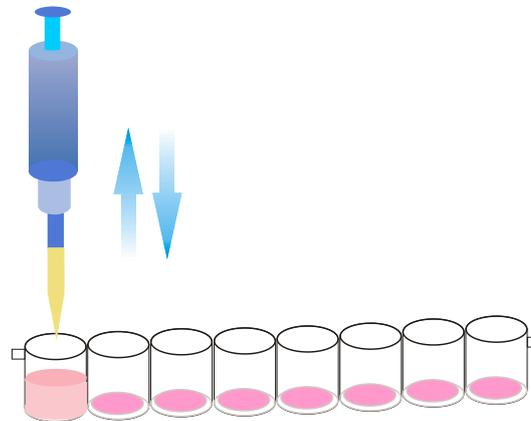
4. Absorb up and down for 5 times to mix sample with reagent completely. Start the timer when the mixture is pink. **Incubate for 5 min.**
