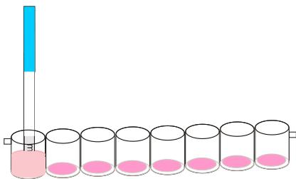
5. Insert the "**MAX**" end of the strip into the mixture; **Incubate for 5min at room temperature again.**
